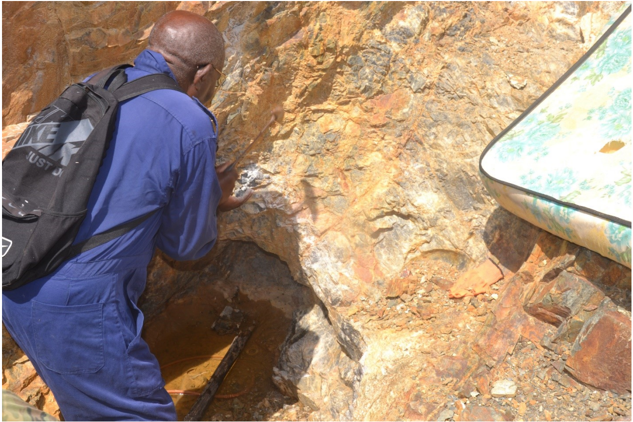
Figure 24: Shear vein at Poeketi (October 6, 2022), Table 4, sample T-02, 0.16 g/t Au
